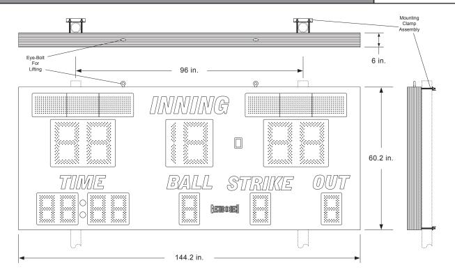
12 ft. x 5 ft., 210 lbs. <u>Electrical Requirements:</u> 3.6 Amps, 120 VAC Display Sizes:
